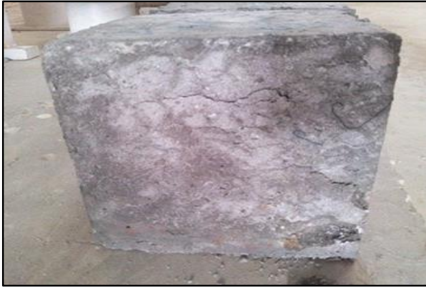
Figure of Testing of Cubes Figure of Cubes after failure under Compression load
