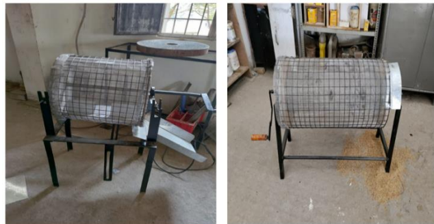
Figure. 1: Photographic view of the finished circular paddy dry model
