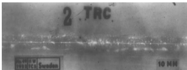
Fig. 14: (a) X-ray image of incomplete penetration flaw is shown. (b) Superimposition of segmented image on original image .It is steel material having thickness ~10mm., metal arc welding process is used for V-shape Butt type welding at down hand position. Radiographic image is taken at 150KV without screen
